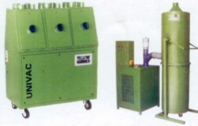
Carding Waste Study Machine and Vacuum Cleaning Machine
